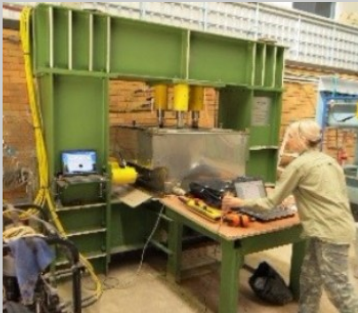
Leonie Bradfield using the large direct shear machine to test the bulk spoil samples at the University of Newcastle.
